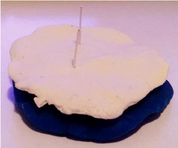
Place the other circle over the insulation and long legs and flip it over. You may need to push the play dough down so the LED tips come through for the eyes. Hook up the black wire to the top piece of conductive play dough and the red wire to the bottom piece of the conductive play dough.
